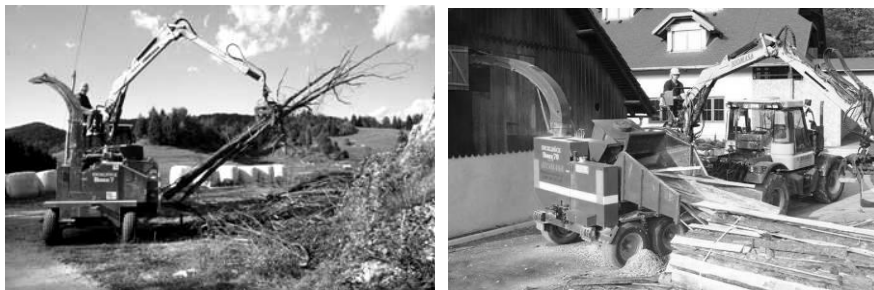
Figure 9. Machines for cutting collected wood biomass.
