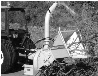
Figure 3. The device for shredding plant mass from plantation of fruit and vineyards.
